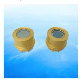
The device is a single four-quadrant or double four-quadrant silicon PIN photodiode module with a built-in preamplifier circuit, which can amplify the weak current signal and convert it into a voltage signal output, realizing the conversion process of "optical-electrical-signal amplification".
