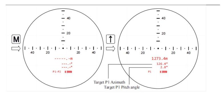
Aim for the second target, press "↑" to complete measurement target P2. Press "↑" again to complete measurement distance between P1 and P2. \* This mode is also suitable for measuring the height of objects.
