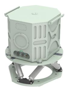
RLG-HX90 inertial navigation system is an inertial navigation system based on type 90 ring laser gyroscope and quartz flexible accelerometer. It can be combined with auxiliary equipment such as GNSS, altimeter, airspeed meter, etc., and can provide air carrier, ground carrier, etc. Navigation information such as speed, position, and attitude.
