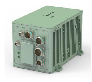
Model 50 inertial navigation system is an inertial navigation system based on type 50 ring laser gyroscope and quartz flexible accelerometer. It can be combined with auxiliary equipment such as GNSS, altimeter, airspeed meter, etc., and can provide air carrier, ground carrier, etc. Navigation information such as speed, position, and attitude.
