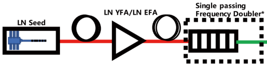
Fig. 1, Schematic of the low noise fiber laser. *The doubler module is equipped with SHG model, for example, LN-YFA-D 及 LN-EFA-D
