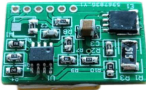
Module is mainly used for pumping and driving 1535nm lasers, and the maximum current can reach 20A.
